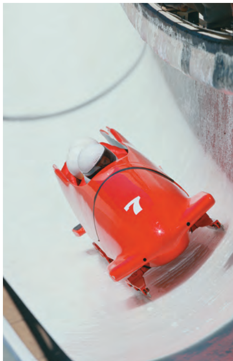
Photo 12.1 As it travels on the curved portion of a track, the bobsled is subjected to a normal component of acceleration directed toward the center of curvature of its path.
