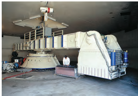
Photo 12.3 The path of specimen being tested in a centrifuge is a horizontal circle. The forces acting on the specimen and its acceleration can be resolved into radial and transverse components with r = \text{constant} .
