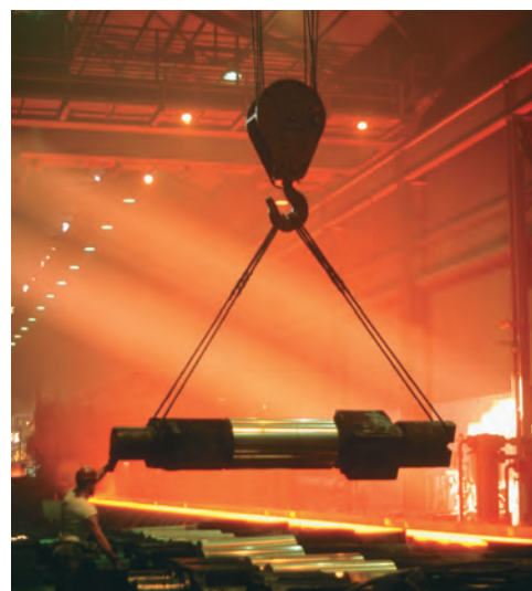
Photo 2.2 As illustrated in the above example, it is possible to determine the tensions in the cables supporting the shaft shown by treating the hook as a particle and then applying the equations of equilibrium to the forces acting on the hook.
