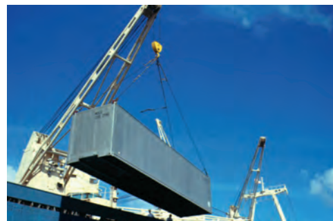
Photo 2.3 While the tension in the four cables supporting the shipping container cannot be found using the three equations of (2.34), a relation between the tensions can be obtained by considering the equilibrium of the hook.
