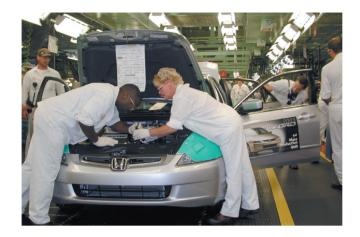
A stage in the assembly line process of producing an automobile where inputs are transformed into outputs. The line is paced as the car moves from one stage to the next after a fixed time interval.
