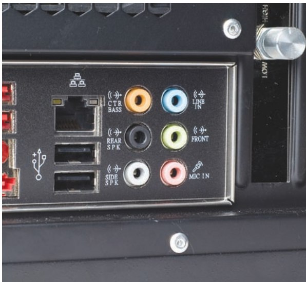
• Figure 3.22 Typical bank of 1/8-inch audio jacks
