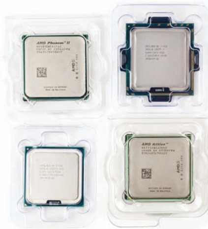
• Figure 3.35 Typical CPUs still in protective packaging
