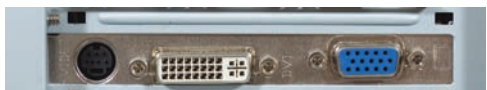
• Figure 3.20 Video card with (from left to right) S-Video, DVI, and VESA ports
