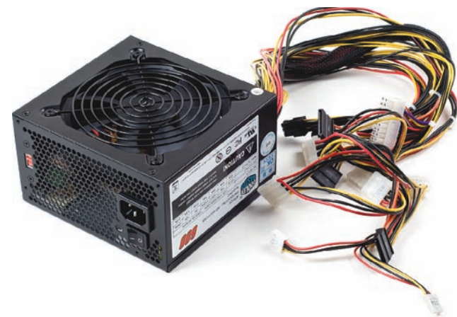
• Figure 3.41 Power supply
