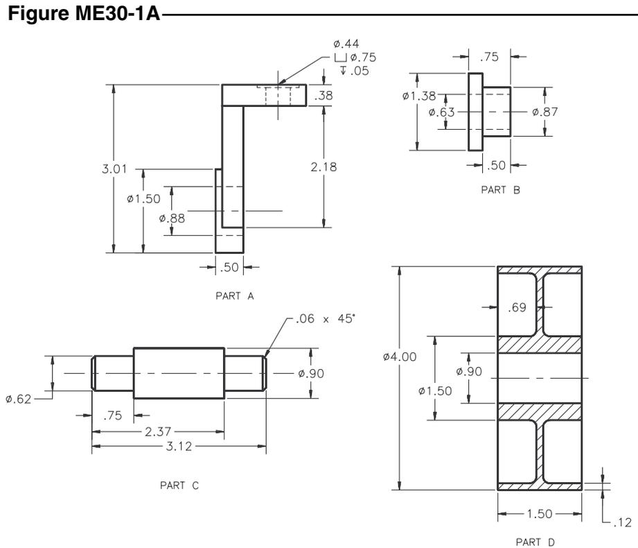
Create a new drawing and use the *Attach* option of the *Xref* command to assemble the individual parts as shown in Figure ME30-1B. *Save* the new drawing as **CH30EX1-M**.
