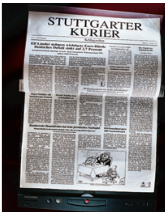
Is this the future of the newspaper? A foldable, updatable, eight-page prototype that uses electronic paper and electronic ink. (Evan Kafka)
