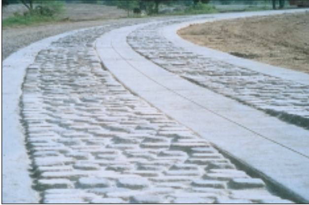
Chrysler's 1.3 mile automated durability track simulates bad roads and is used to test the integrity of automobiles and trucks. Chrysler vehicles are "guided" by computer-controlled robots.
