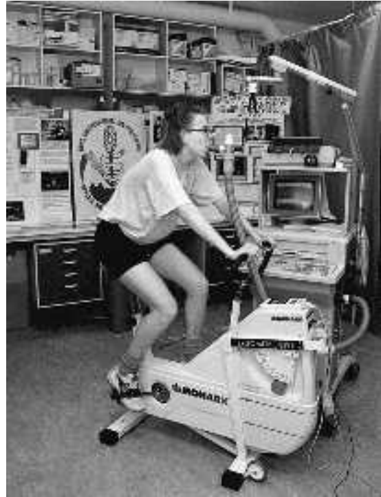
Figure 4-11 Bicycle ergometers are convenient, stationary laboratory devices to control the external work rate (power output) while physiological responses to standardized or experimental protocols are observed. Courtesy of Monark, Inc., Varberg, Sweden.
