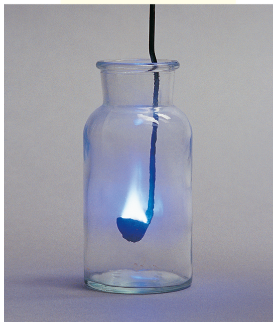
Sulfur burning in oxygen to form sulfur dioxide.
