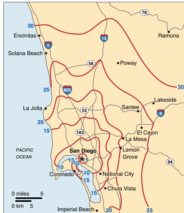
Figure 1.5 Lines of equal travel time ( isochrones : from Greek, isos , equal, and chronos , time) mark off the different linear distances accessible within given spans of time from a starting point. The fingerlike outlines of isochrone boundaries reflect variations in road conditions, terrain, traffic congestion, and other aids or impediments to movement. On this map, the areas within 30 minutes’ travel time from downtown San Diego are recorded for the year 2002. Note the effect of freeways on travel time.
