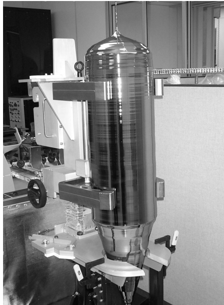
Figure 7.2 | A 300-mm single-crystal silicon boule cooling on a material-handling device.
