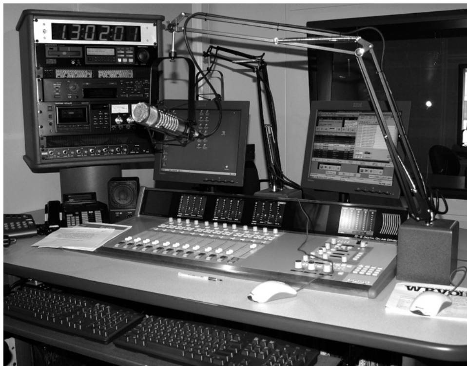
Modern radio production boards use slide faders to control audio levels from various input sources.
