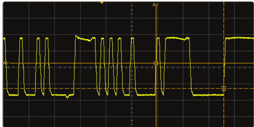
Figure 15. Oscilloscope display correlated to logic analyzer with same trigger point at the SOF
