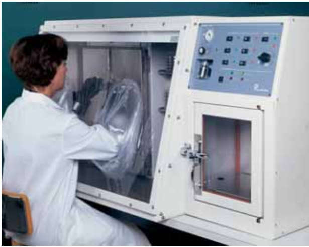
Figure 7.22 An Anaerobic Work Chamber and Incubator. This anaerobic system contains an oxygen-free work area and an incubator. The interchange compartment on the right of the work area allows materials to be transferred inside without exposing the interior to oxygen. The anoxic atmosphere is maintained largely with a vacuum pump and nitrogen purges. The remaining oxygen is removed by a palladium catalyst and hydrogen. The oxygen reacts with hydrogen to form water, which is absorbed by desiccant.
