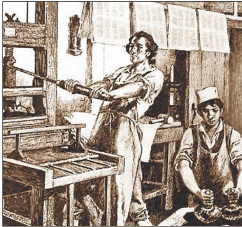
Presses like this were used to print books and newspapers in colonial times. With skill and arm strength, a printer and a “devil” (his assistant) could crank out 200 pages an hour.
