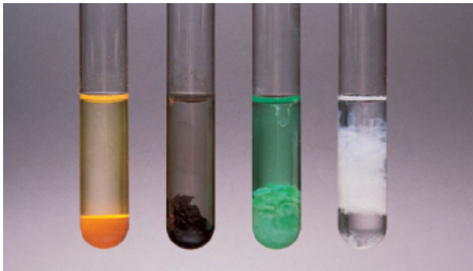
Figure 4.4 Appearance of several precipitates. From left to right: \text{CdS} , \text{PbS} , \text{Ni(OH)}_2 , and \text{Al(OH)}_3 .
