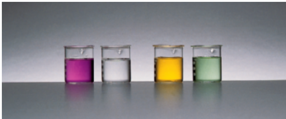
Figure 4.22 Left to right: Solutions containing the \text{MnO}_4^- , \text{Mn}^{2+} , \text{Cr}_2\text{O}_7^{2-} , and \text{Cr}^{3+} ions.
