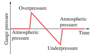
**Figure 12.20** The variation in pressure at a point on the ground as a supersonic plane flies overhead.
