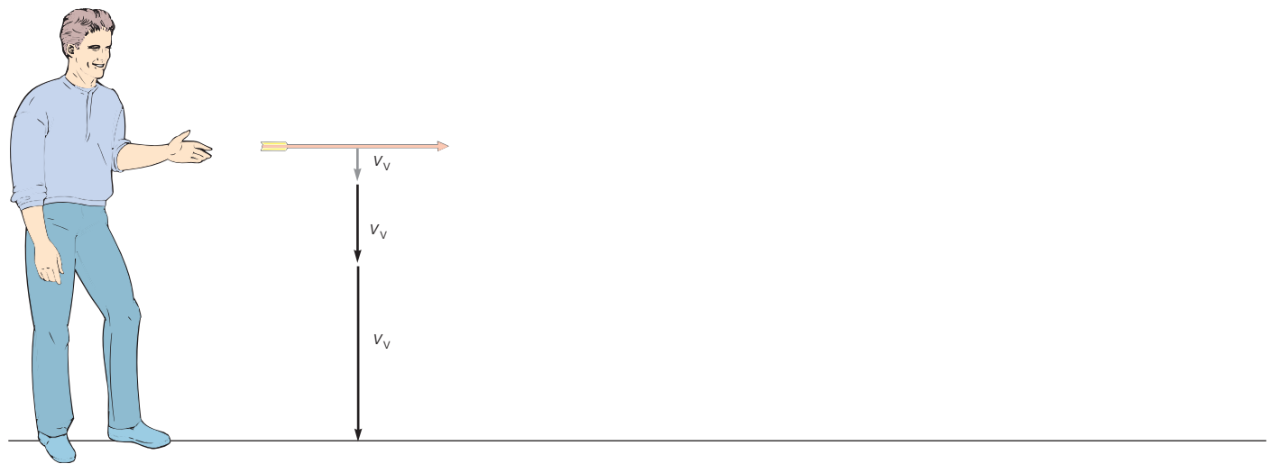
FIGURE 2.12 A horizontal projectile has the same horizontal velocity throughout the fall as it accelerates toward the surface, with the combined effect resulting in a curved path. Neglecting air resistance, an arrow shot horizontally will strike the ground at the same time as one dropped from the same height above the ground, as shown here by the increasing vertical velocity arrows.
