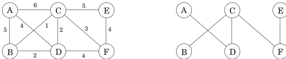
Figure 5.1 The minimum spanning tree found by Kruskal's algorithm.
