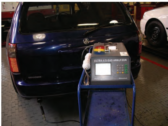
Figure 13.3 An exhaust-gas analyser takes a sample of the exhaust gas and analyses it for emissions
